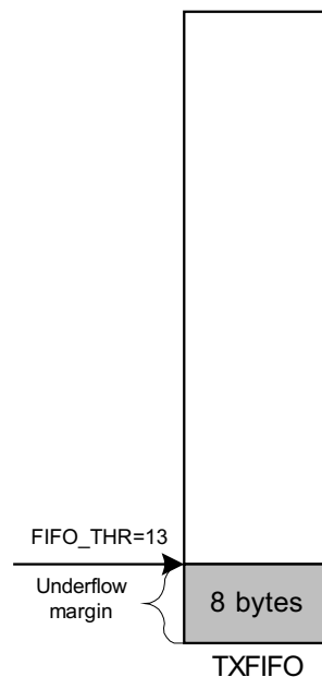
Figure 5-14. Example of FIFO at Threshold
