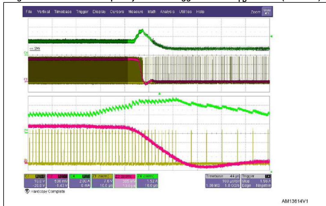
Figure 18. Current and frequency foldback triggered when V_{FB} < 300 \text{ mV} (red trace)
