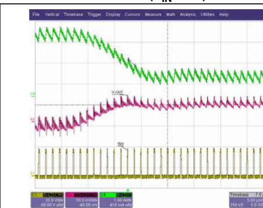
Figure 47. Zoom - 1 A to 3 A falling edge load transient ( V_{IN} 24 V)
