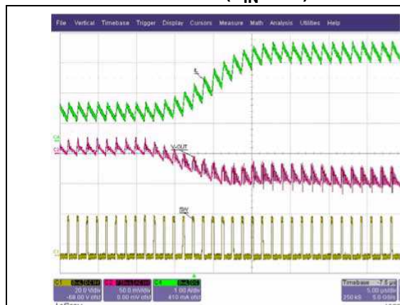
Figure 46. Zoom - 1 A to 3 A rising edge load transient ( V_{IN} 24 V)
