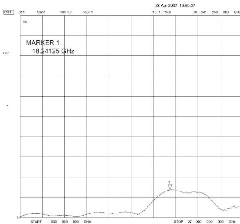
Adapter: HPA152-01 2.92mm/Female-SMA/Female
