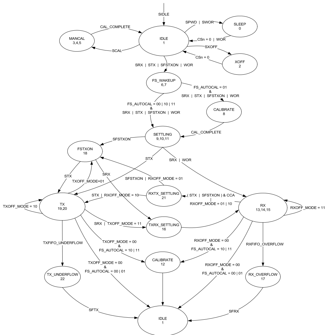
Figure 25: Complete Radio Control State Diagram
